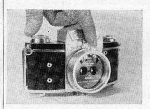
Here's the Kin-Dar Hypo-Stereo attachment on the Exakta. The press button resets the automatic diaphragm to maximum opening after exposure.
