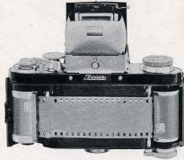
The VX uses economical 35-mm. black-and-white and color film in standard cartridges. Each roll gives you 20 or 36 exposures at a cost per picture only a fraction that of larger sizes. Cartridge-to-cartridge film feed eliminates rewinding and provides rapid, easy operation. Since one short movement of a lever transports the film and cocks the shutter simultaneously, the speed with which a series of pictures can be taken with the Exakta VX is unsurpassed.
