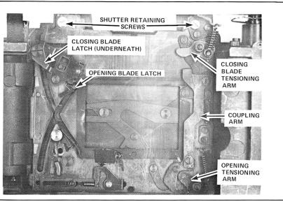
cocking arms may be adjusted if necessary. It will be necessary to adjust this linkage if there is a gap between the blades as they're being cocked, or if one of the blades does not travel far enough to be latched in the cocked position.
