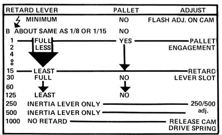
release cam drive spring tension must be changed.
