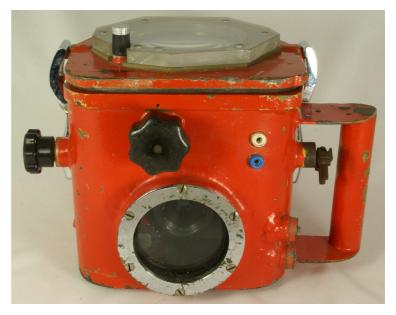
The interior is rusty and stinks, so the seals are clearly not what they ought to be. The focussing mechanism is quite complicated, with five cogwheels and a corrugated iron band around the lens. The first two cogwheels were connected by a chain, but unfortunately that is rusted and broken.
