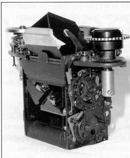
Shutter speed selector wheel with cam behind.
