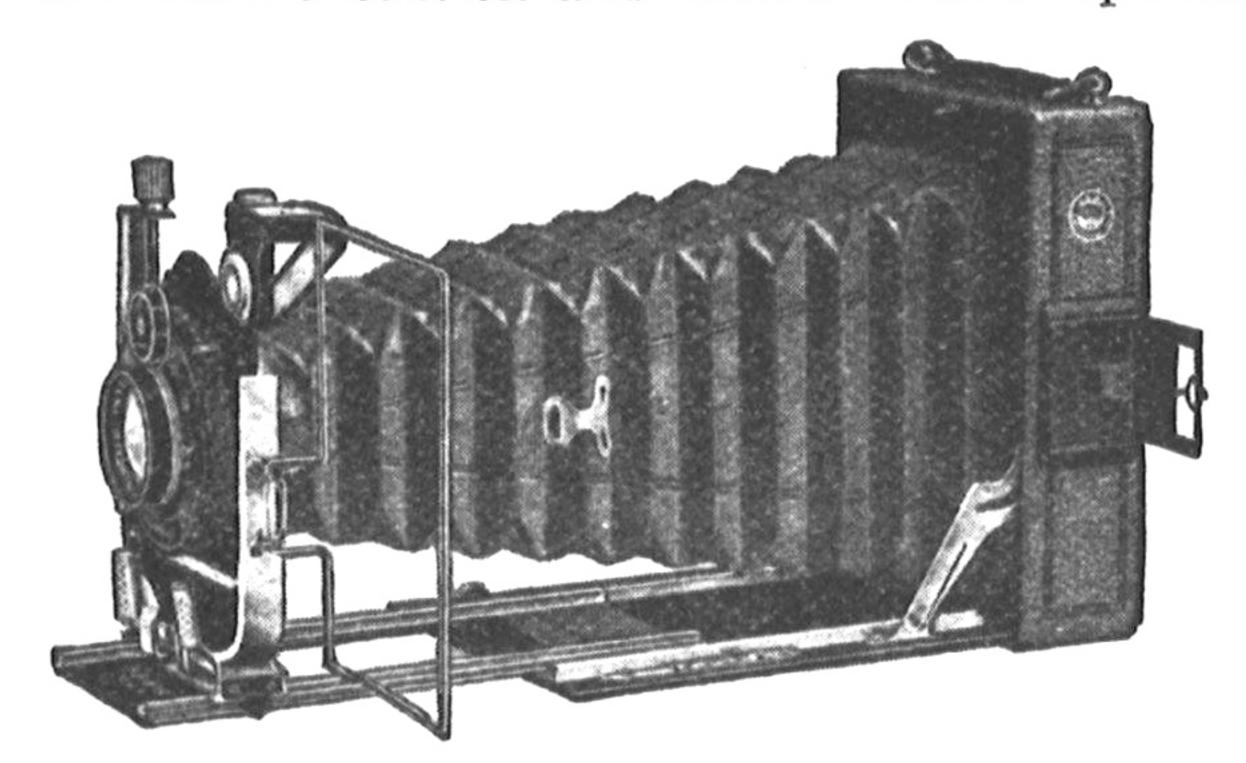
amply sufficing for the fitting of an  $f/3 \cdot 5$  lens of appropriate focal length. Rising front and cross front movements are both operated by screw, and in addition to the reversible brilliant finder there is direct-vision finder for use when taking oblong pictures.
