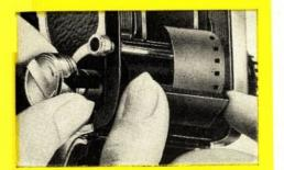
3. Open the camera back. Withdraw the rewind crank (39) by means of its knob, and remove the cassette of exposed film from the camera. Depress the knob on the rewind crank to push
