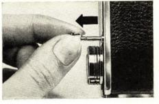
cutting knife (37): Withdraw the knob (38) about 13/4 inches from the camera body. Then press the knob (38), returning it to its rest position. Wind on, and expose two blank frames, in order to draw the end of the film across into the take-up cassette.
