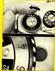
10. Setting frame counter (6). Turn the disc of the frame counter (6) with the index finger to the left (anti-clockwise), until, when using a film with 36 exposures the figure "36", or when using a film with 20 exposures the figure "20" appears in the centre of the window.
