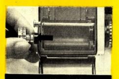
2. Pull out the rewind crank (39) by means of its knob.
