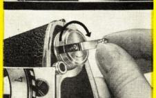
2. Hold the camera in the left hand. Swing out the rewind crank, and with the right hand turn it evenly and slowly in a clockwise direction, until it is felt that it turns more easily. The film has now been rewound. (If the film is rewound at too great a speed, static electricity will cause discharge marks to appear on the negatives.) If the film is being correctly rewound, the indicator disc (20) will show this by revolving also.
