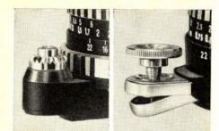
For all exposure times of 1/s sec. or longer, or exposures using the delayed action, lenses having automatic diaphragms should be set to manual in order to avoid premature opening of the aperture. When using the Domiplan 2.8/50 lens, a cable release with a long plunger and time-exposure lock, or the special locking knob (available as an accessory) should be employed for the release rocker. For more information regarding this, see the detailed description of lenses on pages 26–29.
