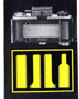
It is not necessary to trim the beginning of the film specially. Any shape of leader can be used with the take-up spool of the EXAKTA VX 1000, either the narrow tongue provided on standard commercial cassettes, or, even better, a straight cut-across end as obtained when cutting lengths of film from bulk rolls. When employing a take-up cassette the film must be trimmed to suit the core of the cassette spool.
