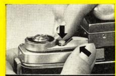
1. Depress the rewind button (9) and secure the rapid-wind lever (8) with a light pressure in the slot of the rewind button, so that it stays in the rewinding position. (The next time that the rapid-wind lever (8) is wound, the rewind button (9) will spring back into its normal position, and the camera would then again be ready for forward transportation of the film.)
