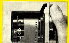
6. Swing the rapid-wind lever (8) right up to its stop (if necessary first releasing the shutter). These two processes may have to be repeated until the teeth of the film-wind sprocket (34) engage with the perforation holes on both sides of the film.
