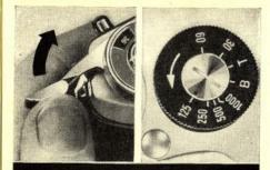
Setting of shutter speeds from 1/1000 sec. to 1/30 sec. (using the delayed action)
