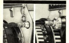
Cable releases (with long plunger) may be screwed into the shutter release knob (3) on the camera or into the release mechanism on the lens (27). This is particularly important when using shutter speeds of 1/a second and slower, and virtually indispensable when employing the B setting. See page 19.
