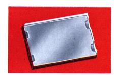
A plane-surfaced ground-glass screen is available for adjusting the image framing without the distraction of a convex focusing lens; this is often useful in copying work, etc. If desired, the focusing screen can be obtained with centimetre or millimetre divisions, right-angle guidelines, etc. The Plane Ground-Glass Screen may be employed in the current Finder Hood, in the Penta Prism and in the Lens Magnifier.
