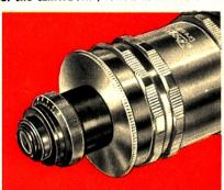
for accepting these lenses. The adapter ring is screwed into the front extension tube. When using the Bellows Attachment the rear bayonet ring is first fitted on the lens carrier, and then the adapter can be screwed into the bayonet ring.
