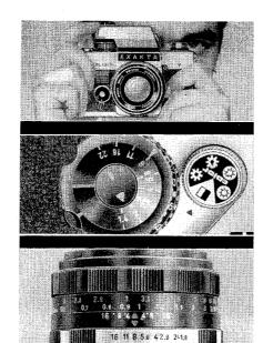
Push the switch (49) to the left. Direct the camera towards the subject to be photographed, and turn the lower disc (50a) of the aperture-setting device until the pointer on the left in the image in the viewfinder will stand in the centre of the circular mark. If the required position of the pointer cannot be obtained, preselect a slower shutter speed.
