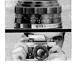
camera towards the subject to be photographed and turn the shutter-speed setting disc (51) until the pointer on the left in the image in the viewfinder will be in the centre of the circular mark. (Do not set intermediate values between the shutter speeds. In case of need effect fine correction by means of the aperture-setting ring (17). If the required position of the pointer cannot be obtained, preselect a smaller aperture number = greater lens aperture.
